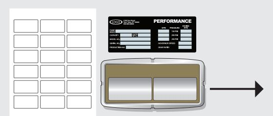
You will start with a blank white peel-off label sheet, a standard plastic overlay with clear windows, and a bezel with a selective adhesive layer applied.
